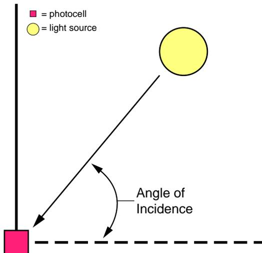
**Figure 1. The Angle of Incidence.** As the angle is increased, the amount of direct light detected is decreased.
