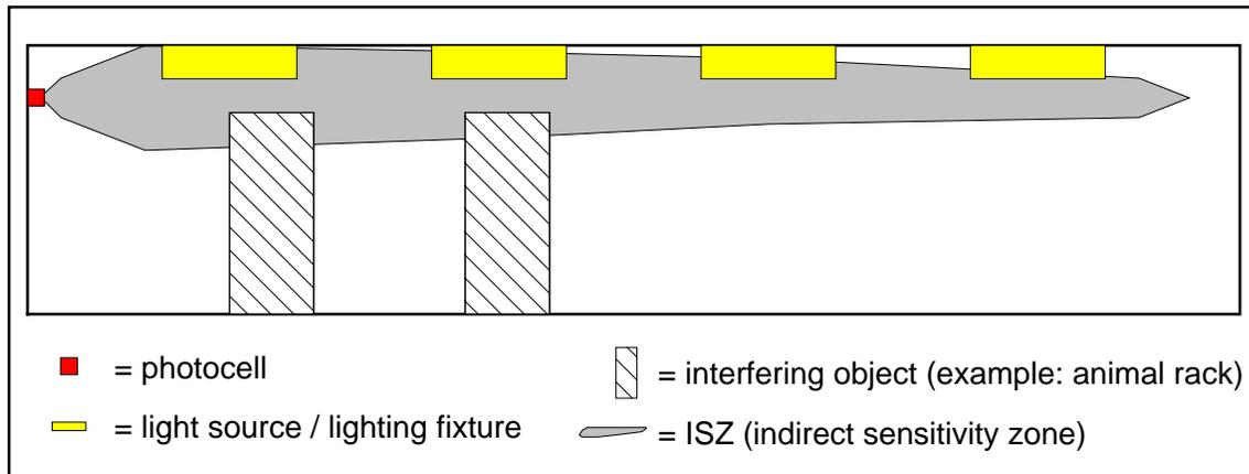
Figure 6. The ISZ for a typical room when the photocell is placed high, near the ceiling. As the position of the photocell is raised, the ISZ becomes smaller.
