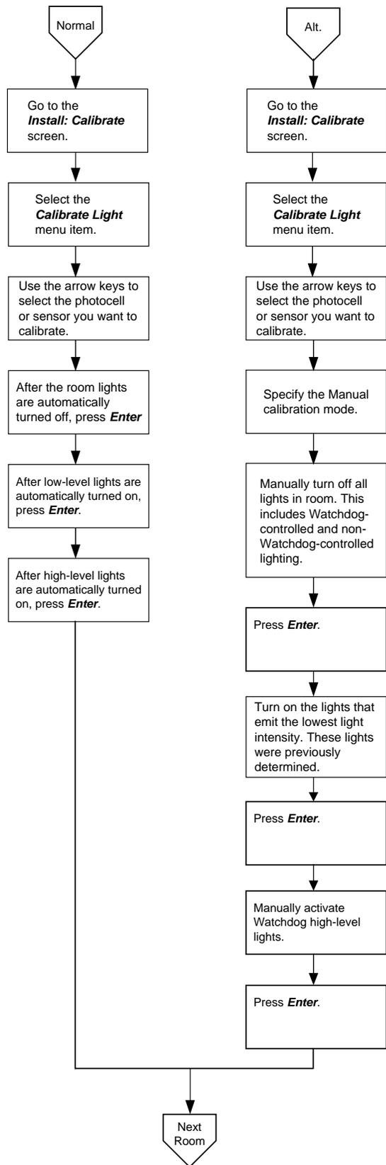
Note: This chart provides an overview of the steps required in calibrating photocells. The exact procedure for performing calibration will vary, depending on the type of equipment in use at a facility. Typically, an ESP or an LCP will be used to perform the calibration. Although the procedures used for both devices are basically the same, there are some minor differences. Detailed instructions can be found in the operating manuals:
