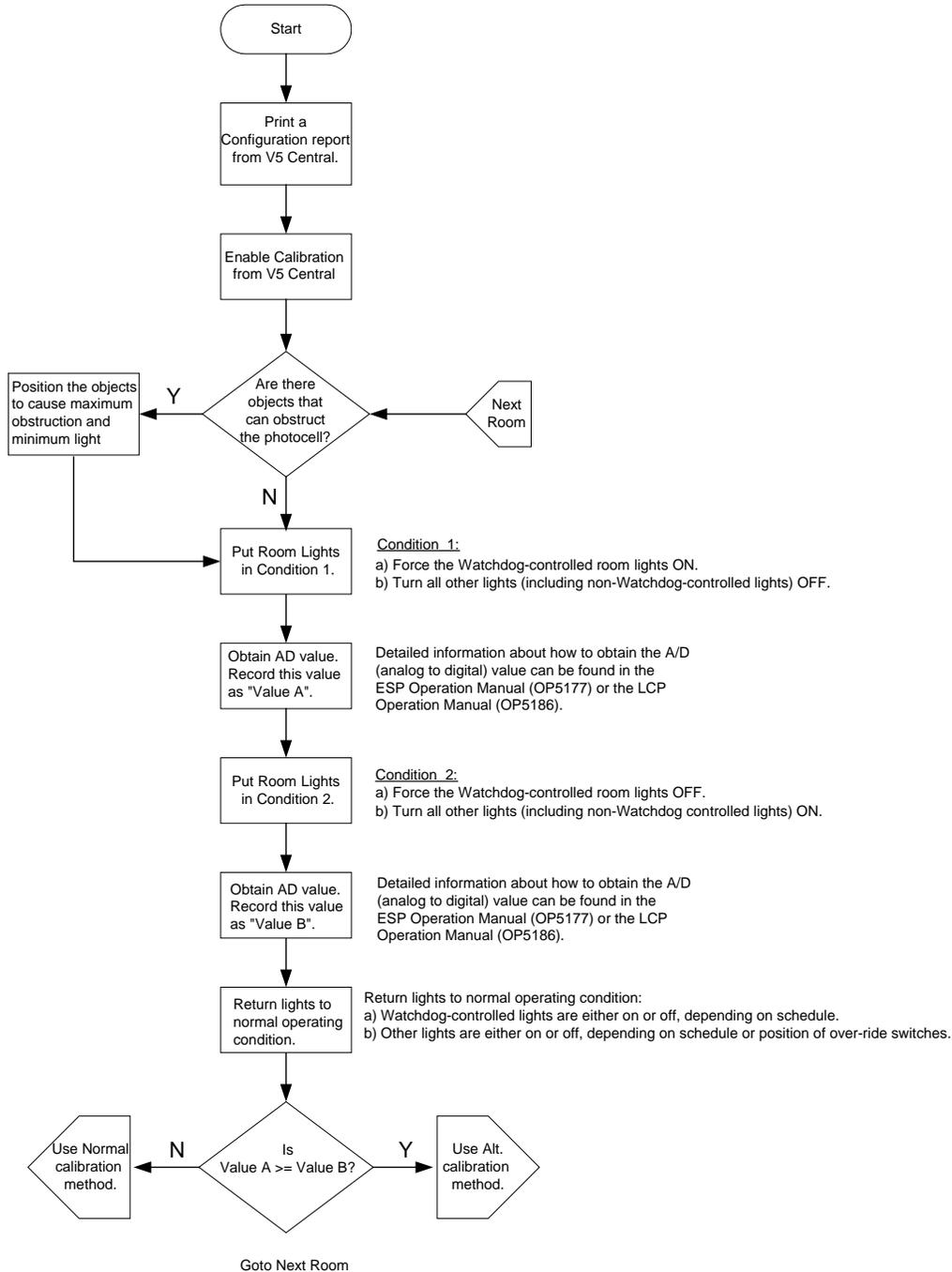
Figure 7. Determining Which Calibration Method to Use.
