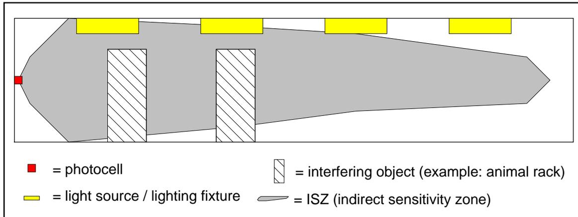
Figure 5. The ISZ for a typical room when the photocell is placed midway between the floor and the ceiling.
