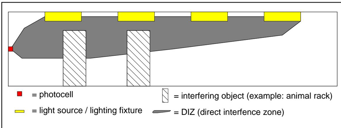
**Figure 3.** The DIZ for a typical room when the photocell is placed midway between the floor and the ceiling.
