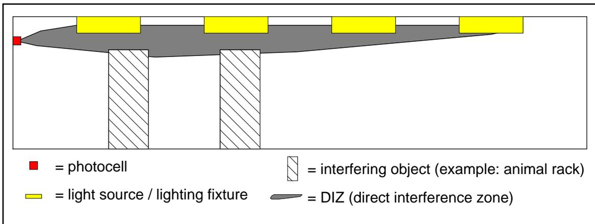
**Figure 4.** The DIZ for a typical room when the photocell is placed high, near the ceiling. As the position of the photocell is raised, the DIZ becomes smaller.
