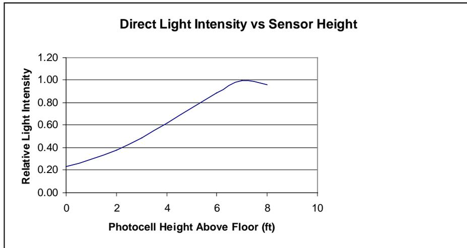
**Figure 2. Where the photocell is placed affects direct light intensity.** More direct light is detected when the photocell is positioned high above the floor. As the photocell is positioned lower, closer to the floor, the angle of incidence is increased and the amount of direct light detected is decreased.
