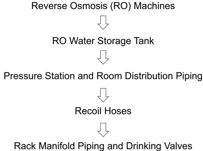
**Figure 1. The components that make up an automated watering system.** All components must be sanitized at regular intervals.
